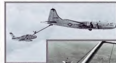
▶ Tanker's eye view ▶ This refuelling method requires the fighter merely to fly straight and level, as the boom operator does all the difficult work from the tanker.
